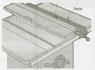
3. Cut the dado (a slot or trench cut into the surface of the board) down the middle of one side of the frame. To do this set the table saw blade to 3/8 of an inch above the surface of the table saw and ½ of an inch from the fence (the fence is shown in the image to the right). Use
